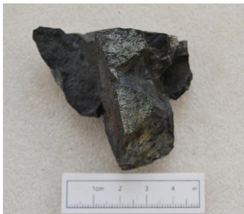
Fig. 17 Typical dolerite from Waterswallows Quarry, Buxton, Derbyshire (photo: Beverley Ballin Smith, GUARD Archaeology Ltd).
